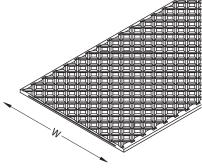
Gantrail pad is normally supplied in 12 metre lengths of the widths shown but is also available in lengths and widths to suit customer specification. This may result in longer lead times – Please contact GANTRAIL for guidance.
